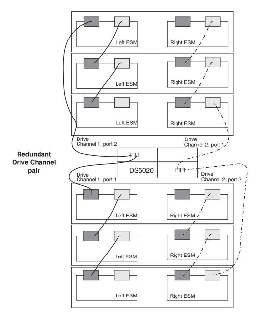
Figure 35. Example of a redundant drive channel pair
